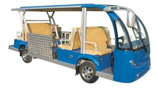
Built based on the electric shuttle bus AMCEG6158K. By removing the third row of seats we have installed a manual ramp.
