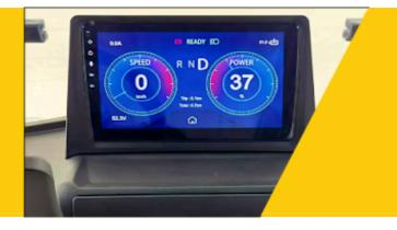
12-inch color LED display. 160° Backup camera, Touch screen for ease of
