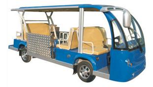
Built based on the electric shuttle bus AMCEG6158K. By removing the third row of seats we have installed a manual ramp.
